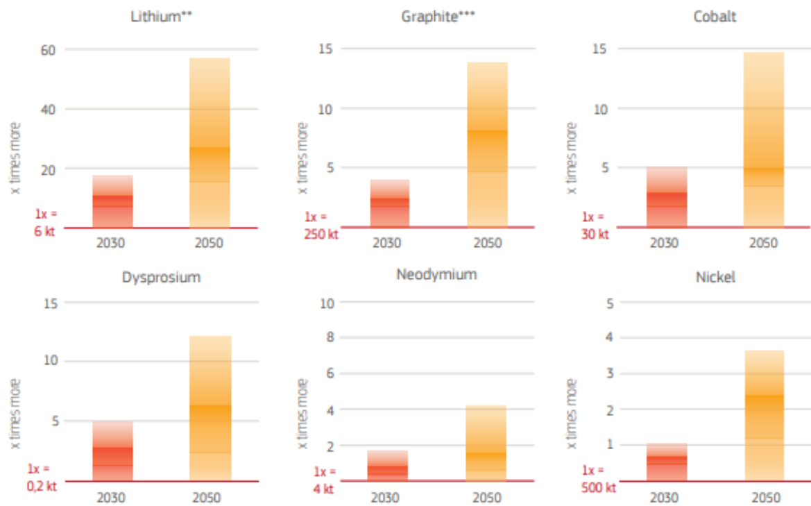
Figure 2: Material consumption for batteries, fuel cells, wind turbines and photovoltaics in 2030 and 2050 as a multiple of current (2020) EU consumption of the material in all applications 211
